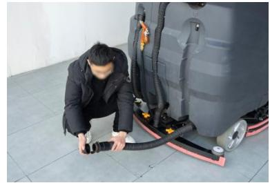
**⚠ Caution :** When flushing the recovery tank, do not splash water into the suction port to prevent the suction motor from burning out.
