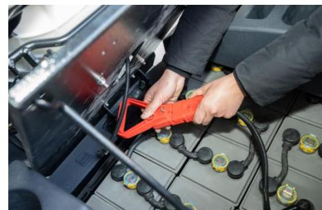
⚠ Caution: Due to the different distances of logistics routes, in order to avoid battery loss during long journeys, the battery cables have been disconnected at the factory.
